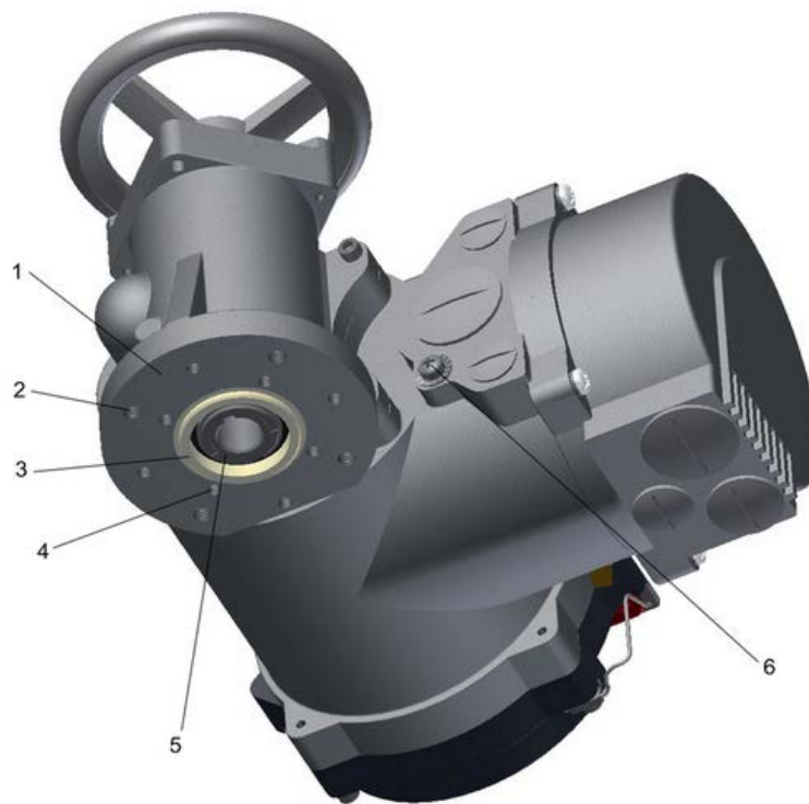
Figure 10: 1... mounting flange, 2... bore pattern G0/F10, 3... centring ring, 4... bore pattern F07, 5... shaft connection, 6... ground connection
